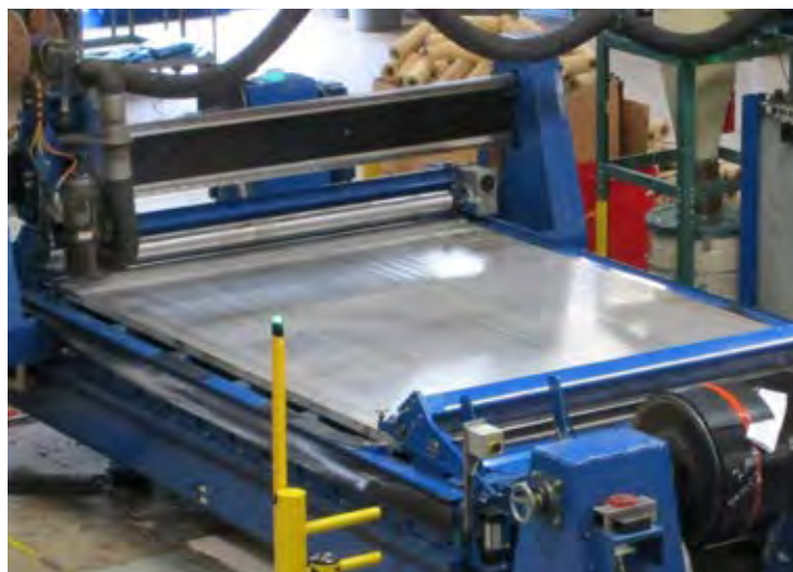
Pregrinder Machine - used in the fabrication of chevron cleated belts.
