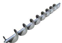
**Helicoid Screws** are manufactured by mounting helicoid flighting on a center pipe and fastening by intermittent welds. Internal collars are inserted in each end and plug welded to accommodate shafts. Screws are structurally reinforced at the ends by end lugs.
