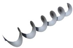
**Helicoid Flighting** is cold rolled from special steel into a continuous helix that produces a work-hardened, smoothly finished flighting surface. Cost-effective helicoid flighting provides superior strength with diameter, pitch and thickness closely controlled.
