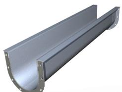
**Angle Flange U-Troughs** are manufactured with structural angle top flanges to provide extra rigidity. End flanges are jig-welded to ensure proper alignment with other trough sections. Angle flange troughs are suitable for light and medium-duty applications.
