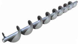
**Rendering Screws** have 3/8-inch thick sectional flights continuously welded on both sides to schedule 80 pipe. 3-bolt drilling is included on both ends.
