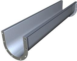
**Rendering U-Troughs** are 3/16-inch thick formed flange troughs with 1/4-inch thick AR-235 wear liners. The wear liners are stitch welded to the troughs for easy removal and replacement.
