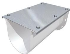
**Trough Covers** are sheared and formed from gauge steel to fit over angle and formed flange troughs. Trough covers provide personnel protection and contain bulk materials being conveyed. Bolts or screw clamps are typically used to fasten covers to troughs.
