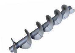
**Sectional Screws** are manufactured by mounting a 360° section of flighting on a center pipe, butt welding each flight together and fastening by intermittent welds. Internal collars are inserted in each end and plug welded to accommodate shafts. Screws are structurally reinforced at the ends by end lugs.
