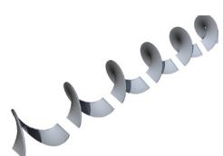
**Sectional Flighting** is manufactured from steel plate and formed into a 360° section of flighting. Sectional flighting is available in heavier thicknesses than helicoid flighting and suitable for more abrasive applications.
