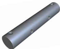
**304 SS Coupling Shafts** are precision cut and drilled to provide an exact fit with helicoid and sectional screws. A space is provided between the screw sections for a hanger and hanger bearing to support additional screw sections.
