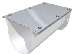
**304 SS Trough Covers** are sheared and formed from gauge steel to fit over angle and formed flange troughs. Trough covers provide personnel protection and contain bulk materials being conveyed. Bolts or screw clamps are typically used to fasten covers to troughs.
