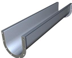
**304 SS Formed Flange U-Troughs** are manufactured with formed top flanges. End flanges are jig-welded to ensure proper alignment with other trough sections. Formed flange troughs are very cost-effective and dust-tight.
