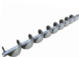
**304 SS Helicoid Screws** are manufactured by mounting helicoid flighting on a center pipe and fastening by intermittent welds. Internal collars are inserted in each end and plug welded to accommodate shafts. Screws are structurally reinforced at the ends by end lugs.
