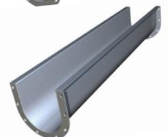
**Formed Flange U-Troughs** are manufactured with formed top flanges. End flanges are jig-welded to ensure proper alignment with other trough sections. Formed flange troughs are cost-effective, dust-tight and suitable for heavy-duty applications.
