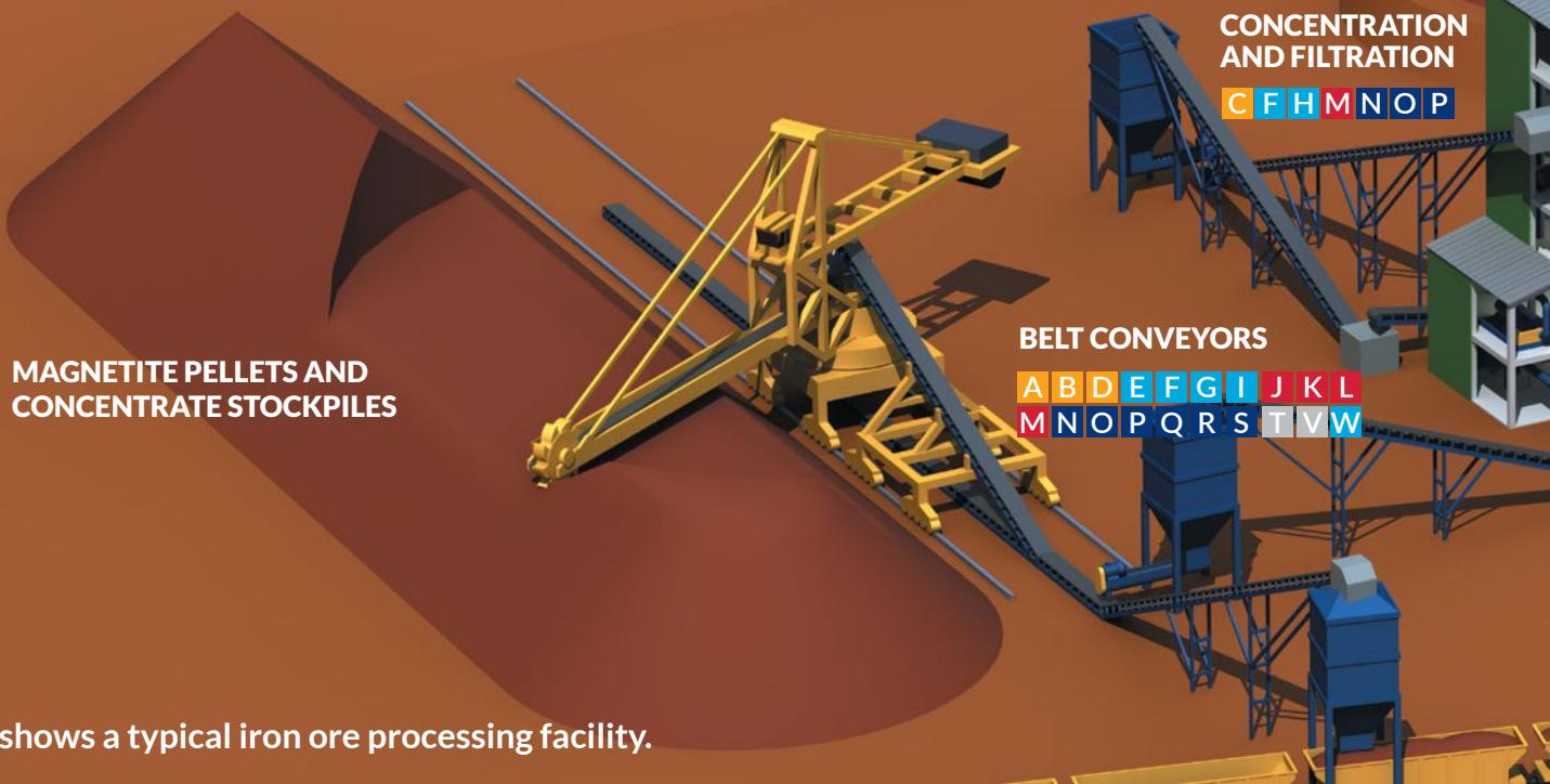
Map shows a typical iron ore processing facility.
