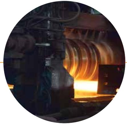
meet your customer's demands for increased productivity, while reducing costs and material waste. Precision bearings – applied to the back-up roll – help ensure strip uniformity by minimizing variations in thickness along the strip's length. For applications where the aesthetic appeal of the strip is important, precision bearings help improve gage accuracy, resulting in a smoother and less wavy finish.
