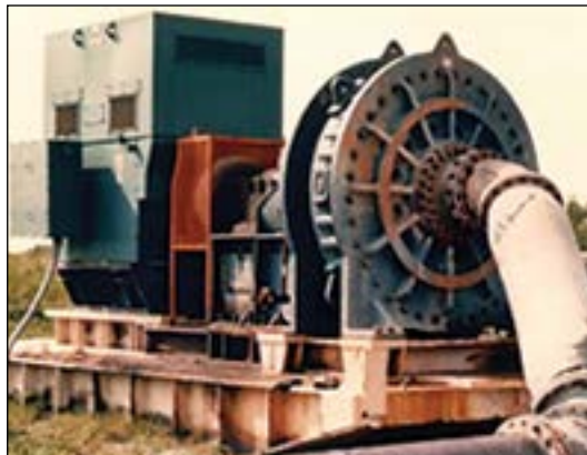
This Excel 1500HP, 514 RPM, 4 kV horizontal motor is powering matrix booster pump in a Florida phosphate mine.
